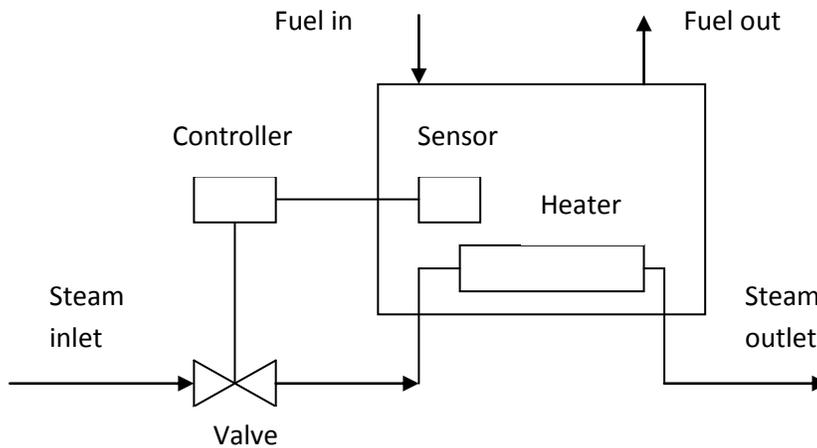
Fig. 1 controlling the viscosity of fuel oil
